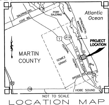
FLORIDA STATE PLANE COORDINATE GEODETIC TIES TO PLAT BOUNDARY BY 3RD ORDER FIELD TRAVERSE UTILIZING MARTIN COUNTY'S HORIZONTAL CONTROL NETWORK STATION MARKS "GS42" & "GS43" REFERENCED TO THE NORTH AMERICAN DATUM OF 1983 ADJUSTMENT OF 1990 (NAD83/90), FLORIDA EAST ZONE (901) UNITS IN U.S. SURVEY FEET. POINT "GIS-A" LOCATION AND VALUES SHOWN ON SHEET 2 OF 7. POINT "GIS-B" LOCATION AND VALUES SHOWN ON SHEET 7 OF 7.
